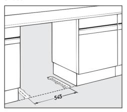
The slides supplied should be used to protect the floor from damage when the machine is pushed into position or taken out for servicing.
